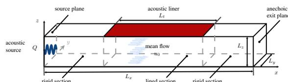
Figure 1. Schematic view of NASA Grazing Incidence Tube (GIT)
