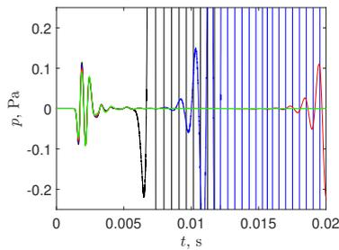
**Figure 2.** Time series of pressure on the rigid wall at  $x = 0.5 L$  for: —  $\epsilon = 1$ , —  $\epsilon = 0.7$ , —  $\epsilon = 0.5$ , —  $\epsilon = 0.3$  and —  $\epsilon = 0$ .
