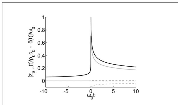
Figure 2. Continuous part of the normalized impulse response  $[z_{S,\infty}(t)/\rho_0 c_0 - \delta(t)]/\omega_0$  as a function of the normalized time  $\omega_0 t$ : (solid line) real and (dashed line) imaginary parts of the first extension (in black) in equation (48) and second extension (in grey) in equation (52) of the Delany and Bazley impedance model of a semi-infinite ground.
