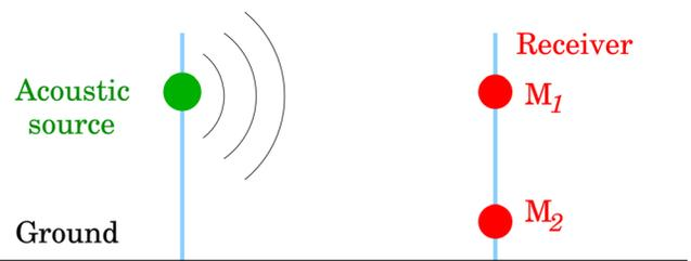
FIG. 4. (Color online) Sketch of the measurement set-up for the transfer function method.
