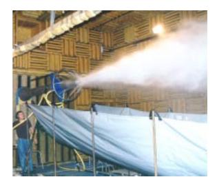
Figure 1 : Injection of water in a supersonic air-jet to reduce the generated noise (Mach=1.3)
