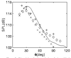
Figure 3 : Directivity of noise emission of a jet at Mach 0.9 (- numerical simulation, Re=65000; x experimental data, Re=3600, + and diamonds, Re=5 10<sup>5</sup>). see ref. [8] for details
