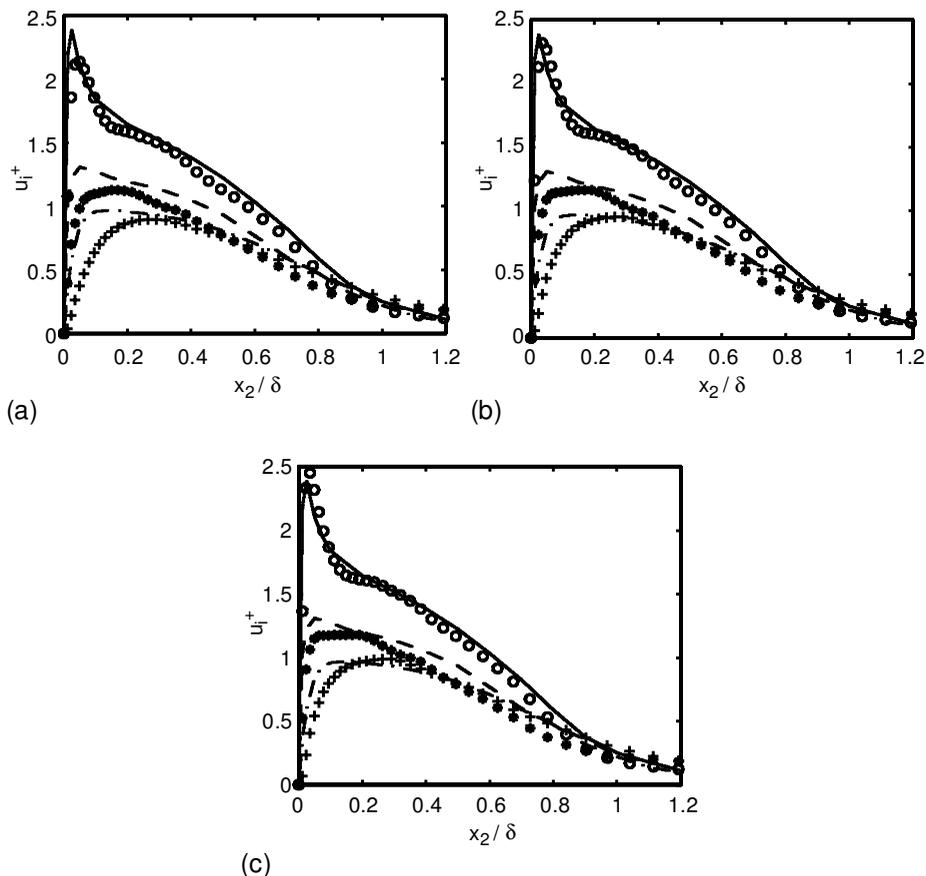
**Figure 4.** Turbulent boundary layer testcase. Turbulent intensities for the spatial LES (symbols) and the temporal DNS of Spalart<sup>29</sup> (lines): ( $\circ \circ$ , —),  $u_{1rms} / u_\tau$ ; ( $++$ , -.-.),  $u_{2rms} / u_\tau$ ; ( $**$ , ---)  $u_{3rms} / u_\tau$ . Three values of the Smagorinsky constant are tested:  $C_s = 0.18$  (a),  $C_s = 0.1$  (b), and  $C_s = 0.02$  (c).
