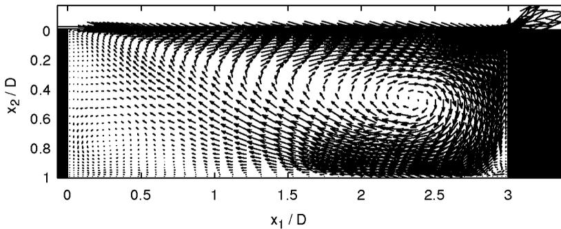
**Figure 11.** Distribution of averaged velocity inside the cavity in the median plane.
