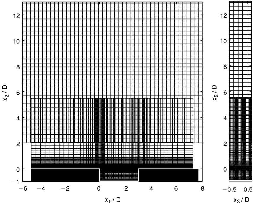
**Figure 5.** Superimposition of the meshgrids used for the DNC (bottom) and for the WNLEE calculation (top). The grids are shown every other four points (sideview on the left and crossview on the right).
