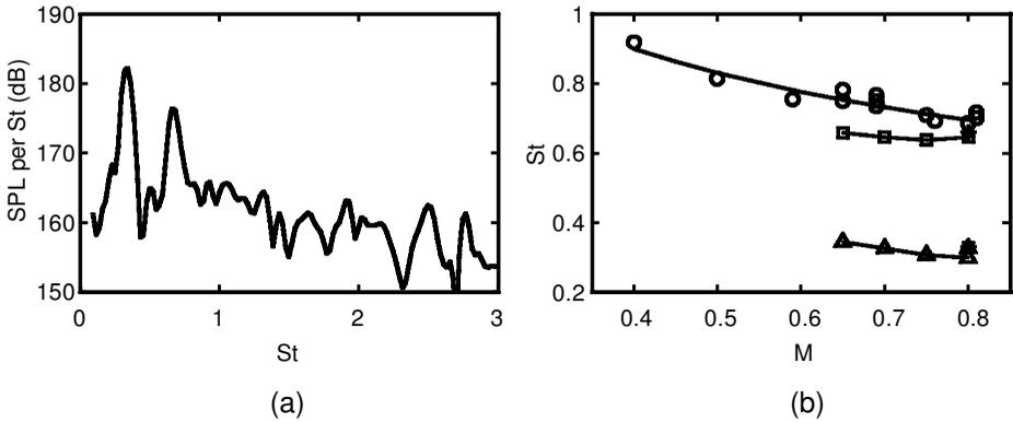
**Figure 6.** (a): Spectrum of the fluctuating pressure near the impingement corner at  $x_1 = L$ ,  $x_2 = 0.02D$ ,  $x_3 = 0$ ; (b): Strouhal number for the principal frequencies versus the Mach number. Comparison between Karamcheti's experiments<sup>1</sup> ( $\circ$  with laminar inflow;  $\square - \Delta$  high and low components with turbulent inflow) and the present simulation ( $*$ ) for a turbulent inflow and  $M = 0.8$ .
