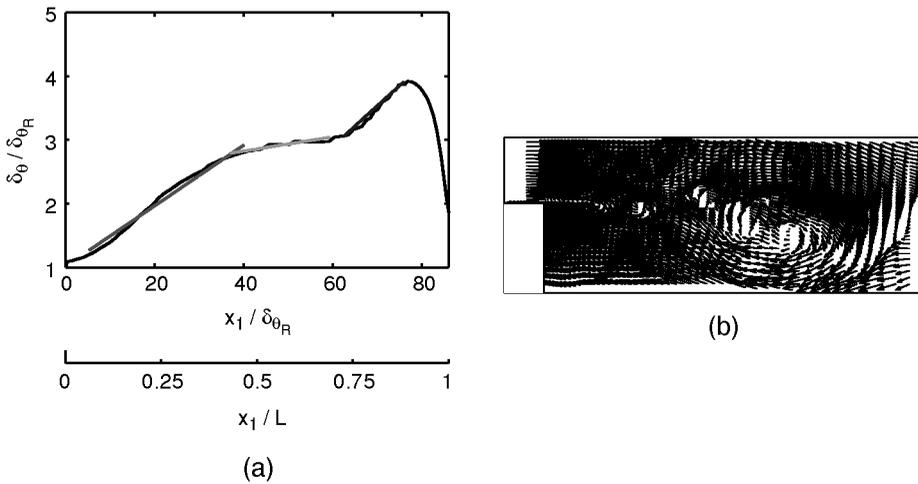
**Figure 9.** (a): Non-dimensional momentum thickness  $\delta_\theta / \delta_{\theta_R}$  between the two corners of the cavity; (b): Zoom of velocity field around the upstream corner of the cavity ( $-0.1 < x_1 / D < 1.1$ ) showing the collective interaction.
