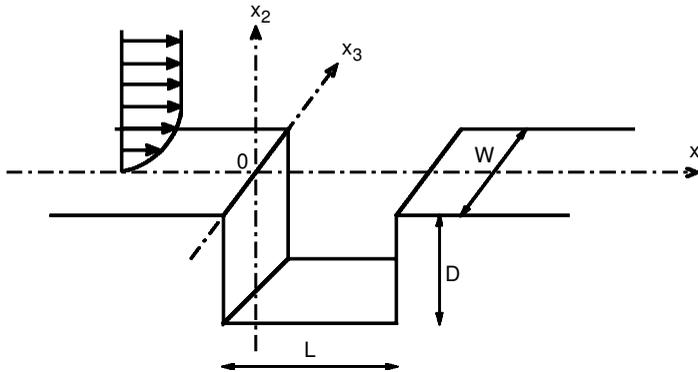
**Figure 1.** Sketch of the flow domain and coordinate system.
