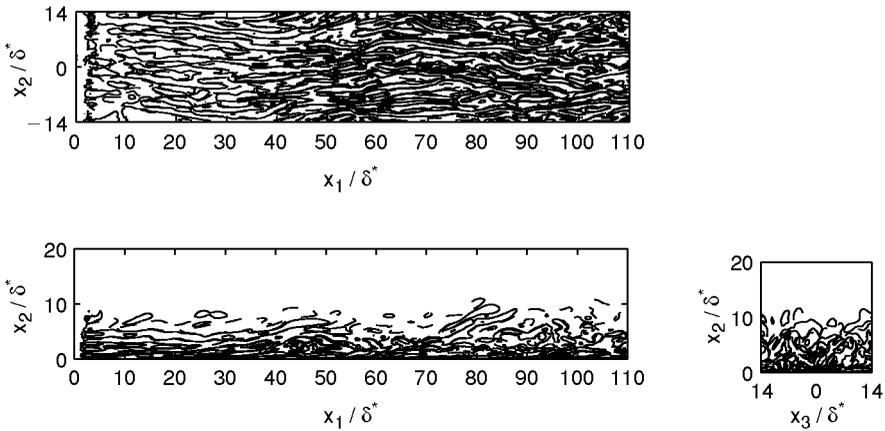
**Figure 2.** Turbulent boundary layer testcase. Vorticity isocontours: topview of  $\omega_{13}$  at  $x_2 = 0.6\delta^*$ , sideview of  $\omega_{12}$  at  $x_3 = 0$ , and crossview of  $\omega_{23}$  at  $x_1 = 86\delta^*$ . (—): positive contours  $[0.1; 1; 10] \times 10^5$ ; (---) : negative contours  $[-10; -1; -0.1] \times 10^5$ .
