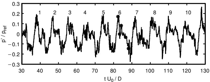
**Figure 7.** Time trace of the fluctuating pressure near the impingement corner at  $x_1 = L$ ,  $x_2 = 0.02D$ ,  $x_3 = 0$ .
