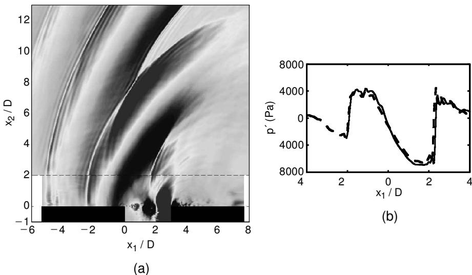
**Figure 13.** (a): Pressure field obtained by the extrapolation method from the extrapolation surface (shown by the dashed line). The DNC near-field is plotted under the extrapolation surface. Sideview in the median plane. Levels between  $-5000$  and  $5000$  Pa; (b): Longitudinal pressure profiles along  $x_2 \approx 3.6D$ . (—), DNC and (---), WNLEE.
