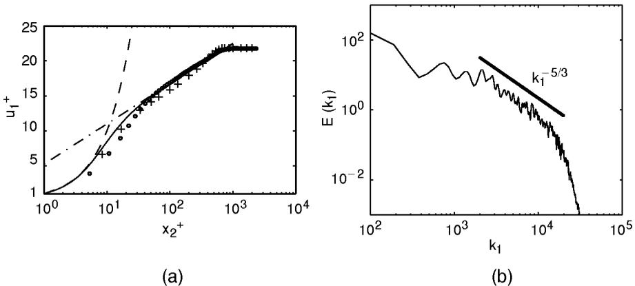
**Figure 3.** Turbulent boundary layer testcase. Mean profile of  $\bar{u}_1/u_\tau$  (a): ( $\circ \circ$ ), present LES; ( $++$ ), Spalart's DNS<sup>29</sup>; (---), linear law; (- . - .), logarithmic law; (—), analytical Van Driest profile. Energy spectrum of vertical velocity fluctuations (b) in the boundary layer at a distance of  $0.5\delta$  from the wall.
