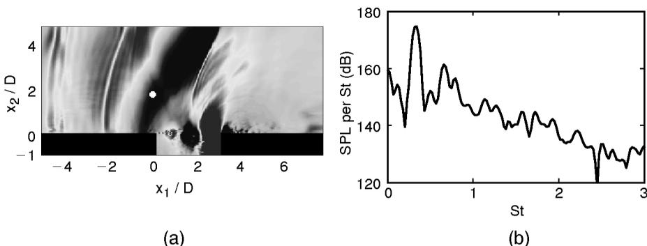
**Figure 12.** (a) Pressure field from the DNC in the midplane of the cavity (levels between  $-5000$  and  $5000$  Pa); (b) Spectrum of pressure fluctuations at the location indicated by a bullet on the left.
