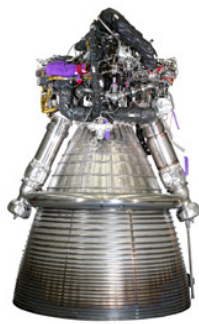
Figure 1.1: The Vulcain 2 engine, manufactured by Snecma. The supersonic flow is accelerated in the diverging nozzle
