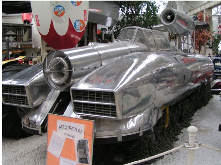
Figure 1.12: Aérotrain developed by Jean Bertin and used by Snecma engineers for flight effect measurements in the 1970's [25]
