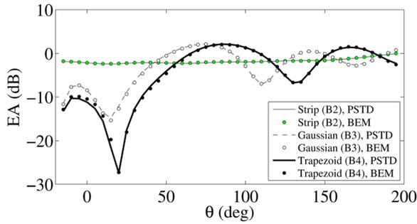
FIG. 9. (Color online) Excess attenuation for the three configurations (B) with  $Z_n = 17.9$  as a function of the receiver position for  $f = c/8\Delta$ . Heights of the Gaussian shape and the trapezoid is  $3\Delta$ .
