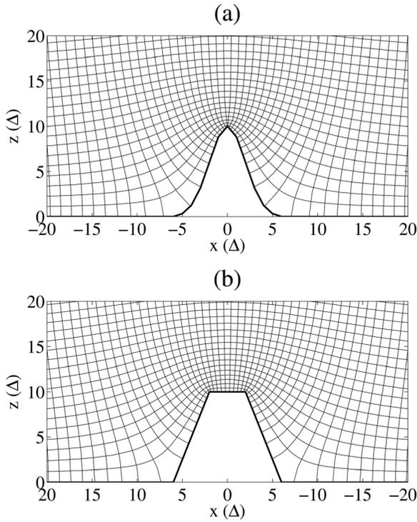
FIG. 5. Mesh close-up around a (a) Gaussian shape and (b) trapezoid, with (thick) modelled geometry (thin)  $u_y$ -mesh.
