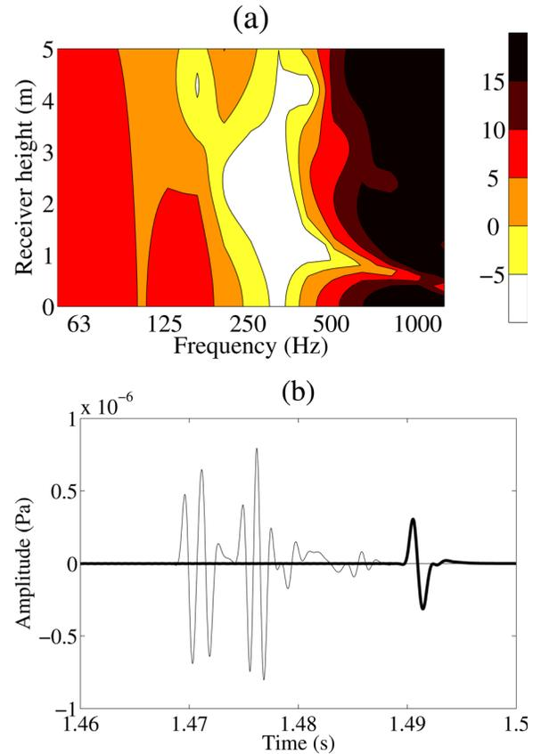
FIG. 11. (Color online) Results for configuration (C). (a) Excess level  $\Delta L_{p,n}$  due to the nocturnal boundary layer (NBL) as a function of 1/3 octave band and receiver height, (b) computed impulse responses at receiver position (500 and 0 m). Results are calculated for sound propagation in an homogeneous atmosphere and in a NBL (thick and thin line, respectively).
