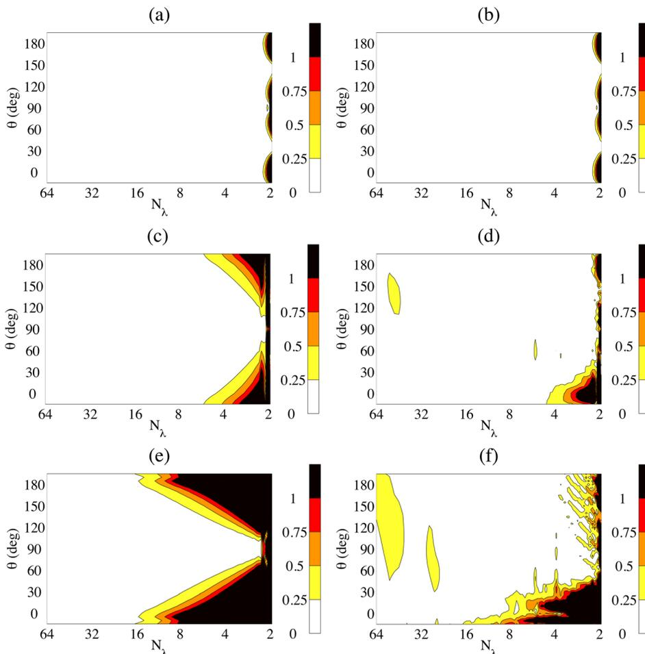
FIG. 4. (Color online) Results for configuration (left), (B1) and (right) (B2).  $\Delta L_{p,n}$  (dB) as a function of the receiver position and  $N_\lambda$  for [(a), (b)]  $Z_n = \infty$ , [(c), (d)]  $Z_n = 17.9$ , [(e), (f)]  $Z_n = 2.6$ .
