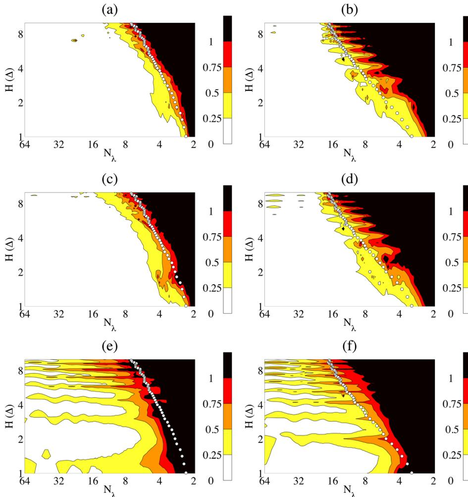
FIG. 6. (Color online) Results for configuration left, (B3) and right, (B4).  $\overline{\Delta L_p}$  results for grid spacing  $\Delta$  as a function of the Gaussian shape or trapezoid height  $H$  and  $N_\lambda$  for [(a), (b)]  $Z_n = \infty$ , [(c), (d)]  $Z_n = 17.9$ , [(e), (f)]  $Z_n = 2.6$ .
