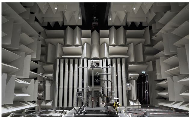
Figure 8. Internal view of the anechoic chamber and of the exhaust sections of the subsonic and supersonic wind tunnels.
