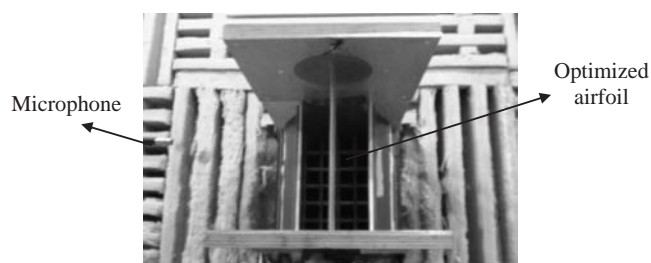
Fig. 4—Experimental facility in the anechoic chamber; wind tunnel-optimized airfoil configuration.
