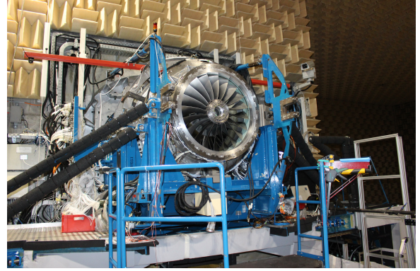
(b) UFFA front view with no inlet.
