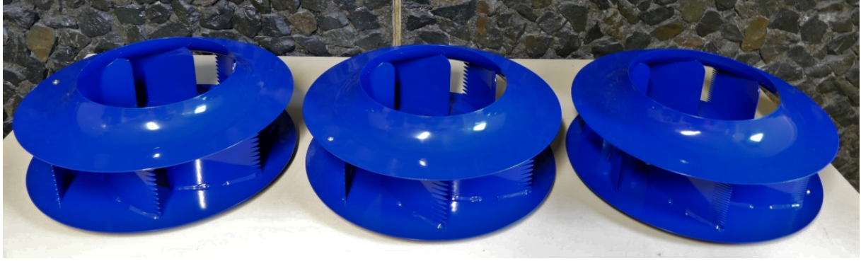
Figure 1.44 – Impeller prototypes with trailing-edge serrations
