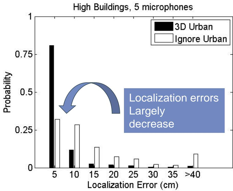
The method is efficient, including in NLOS
