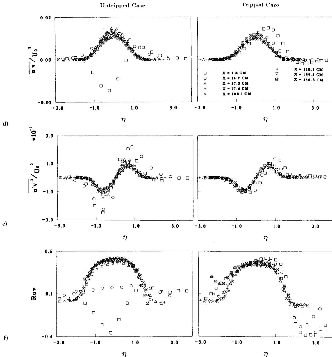
Fig. 4 (continued) Profiles of turbulence products in similarity coordinates, at different streamwise stations. Case with untripped initial boundary layers is on the left, tripped initial boundary layers on the right. d) primary shear stress,  $u'v'$ , e) primary shear stress transport,  $u'v'^2$ , f) shear correlation coefficient,  $R_{uv}$ .
