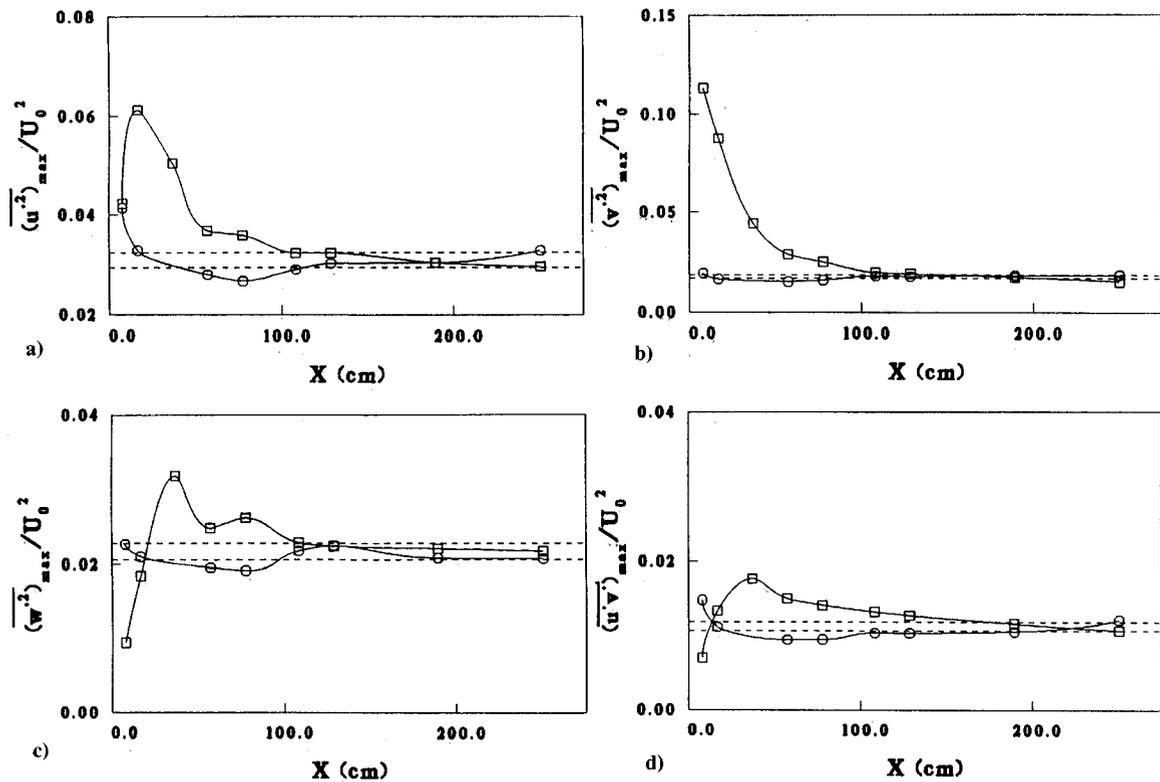
Fig. 5 Streamwise development of maximum level of turbulence products.  $\square$ : untripped initial boundary layers,  $\circ$ : tripped initial boundary layers, ---  $\pm 5\%$  range around measured asymptotic level. a) streamwise normal stress,  $u'^2$ , b) cross-stream normal stress,  $v'^2$ , c) spanwise normal stress,  $w'^2$ , d) primary shear stress,  $u'v'$ .
