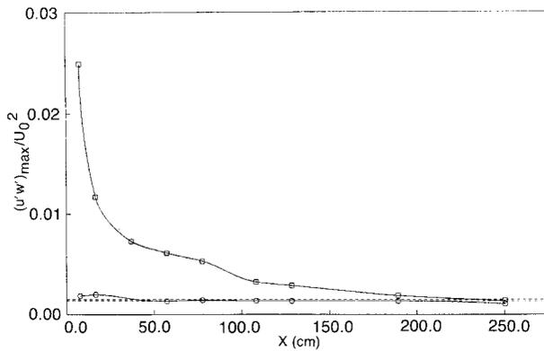
Fig. 7 Streamwise development of maximum level of secondary shear stress,  $\overline{u'w'}$ .  $\square$ : untripped initial boundary layers,  $\circ$ : tripped initial boundary layers, ----  $\pm 5\%$  range around measured asymptotic level.
