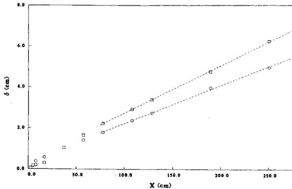
Fig. 3 Growth of mixing layer with increasing streamwise distance;  $\square$ : untripped initial boundary layers,  $\circ$ : tripped initial boundary layers.
