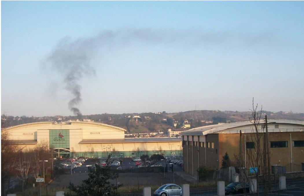
Smoke plume in the presence of a near surface temperature inversion, which hinders vertical turbulent motion and drives the plume horizontally. *The Quays Shopping Centre*, near to Tiur and Cloghoge, taken by Eric Jones (Bailly & Comte-Bellot, 2015)
