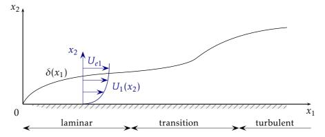
Development of a zero-pression-gradient boundary layer on a flat plate. The transition occurs for  $\text{Re}_{x_1} = x_1 U_{e1} / \nu \simeq 3.2 \times 10^5$ , that is  $\text{Re}_{\delta} = \delta U_{e1} / \nu \simeq 2800$ .
