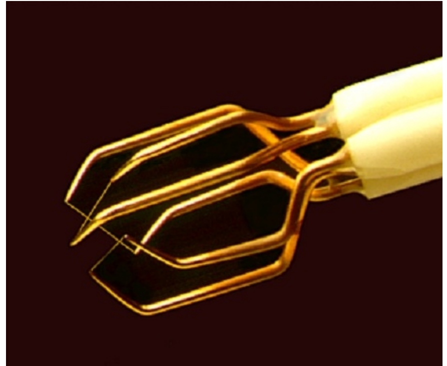
Tri-axial probes for 3-D flows : 3 sensors in an orthogonal system, measures within 70^\circ cone (image from Dantec)
