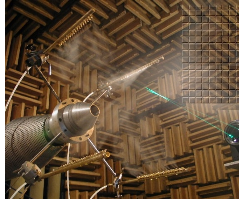
LDV measurement in a free subsonic jet in the anechoic wind tunnel (V. Fleury & S. Barré, LMFA)
